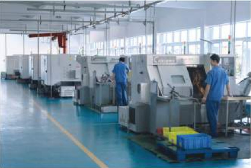
CNC lathes for turning operations
