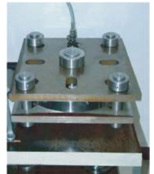
High pressure test rig of ADP Hydraulic nut
