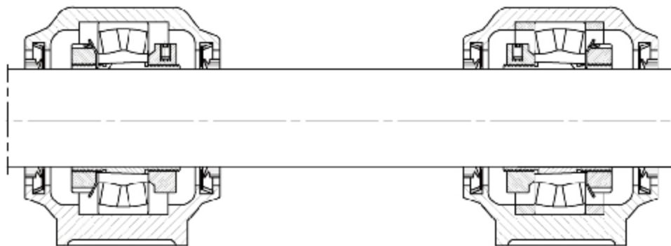
Typical application of ADP easy extraction adapter sleeves, mounted on smoothing shaft without space problems.
