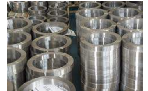
Forged-steel rings for large-sized lock nuts
