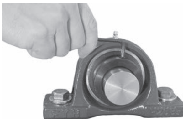
Fig. 14.10 Installing eccentric locking collar
