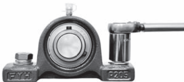
Fig. 14.4 Installation of set screw units
