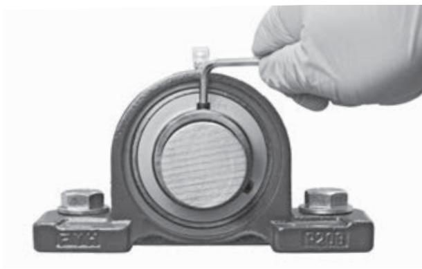
Fig. 14.5 Tightening of set screws
