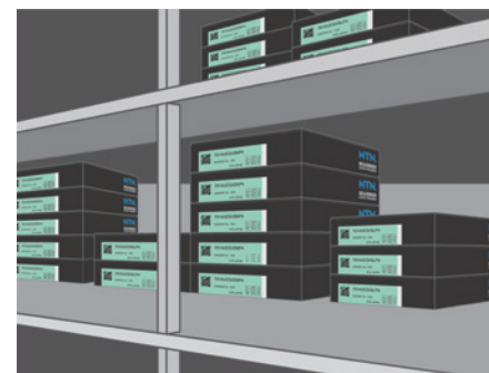
Fig. 6.37 Storing one-bearing boxes on a shelf
